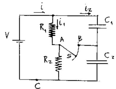
$$C_1, C_2 \text{ son dos capacitores en serie} \rightarrow C_e = \frac{1}{\frac{1}{C_1} + \frac{1}{C_2}}, \quad Q_1 = Q_2 = Q \Rightarrow V = Q \left( \frac{1}{C_1} + \frac{1}{C_2} \right)$$
