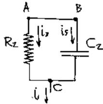
$$\begin{aligned} -i_2 R_2 + \frac{Q_2}{C_2} &= 0 \\ -i_3 R_2 + (V_B - V_C) &= 0 \\ V_B - V_C &= i_3 R_2 \end{aligned}$$
