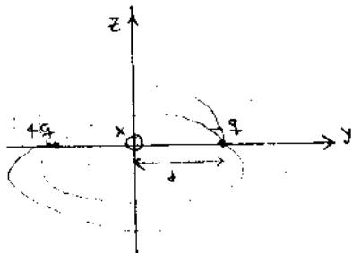
$$V(x, y, z) = k \cdot \frac{q}{\sqrt{x^2 + (y+d)^2 + z^2}} + k \cdot \frac{-q}{\sqrt{x^2 + (y-d)^2 + z^2}}$$
